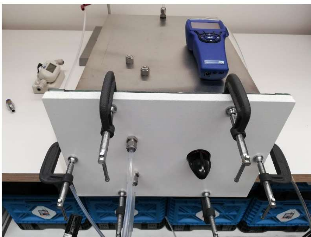
Environmental chamber showing MAGdrain installation
